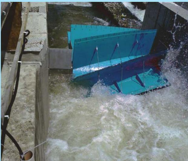
**Fig. 5.** Inflow and air entrainment upstream of the HPM
