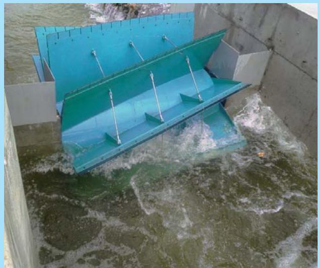
**Fig. 6.** Immersion of the HPM wheel blades at low upstream water level
