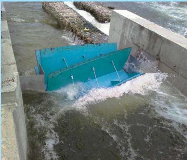
**Fig. 3.** Water inflow between the HPM blades and curvature of the upstream water surface
