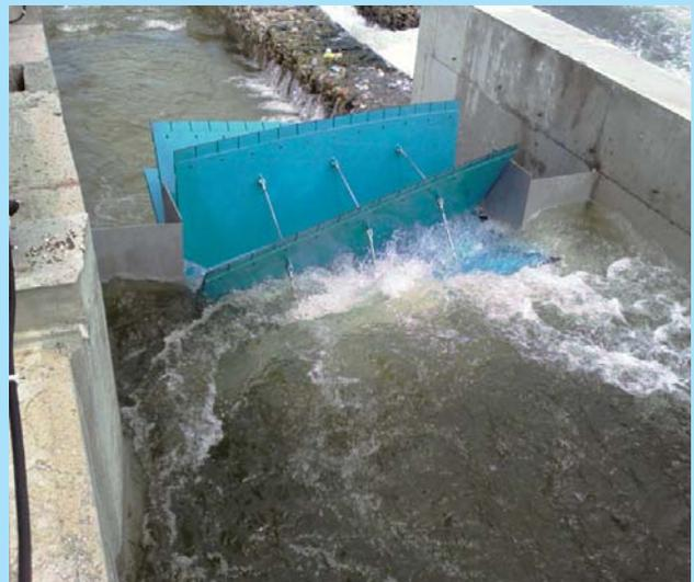
**Fig. 4.** Water inflow conditions between the blades of the HPM wheel
